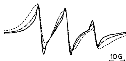
FIGURE 8 ESR spectra for DPPC liposomes containing various amounts of SL9-eggPA. SL9-eggPA was incorporated into liposomes composed of DPPC and DCP (molar ratio 1:0.1) in the amounts of 5.5 mol% (—), 18.9 mol% (---), and 48.2 mol% (···). The concentration of DPPC was 10 mM. The relative amplifications for the spectra were 5, 2, and 1 for 5.5, 18.9, and 48.2 mol%, respectively. The spectra were measured at 25°C as described in the legend to Fig. 2.
